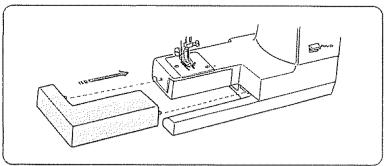
To Attach the Extension Table (for flat-bed sewing)
